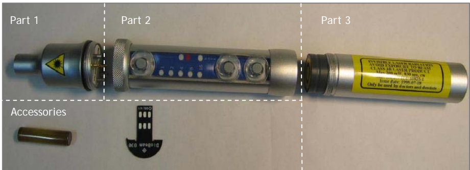
Illustration 2: Laser taken apart consisting of: Part 1: Laser head, with laser diode build in and sealed. Part 2: Control part. Part 3: Battery part. Accessories: Light tip and coded key.
